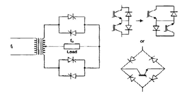
A positive center-tap thyristor converter is connected in anti-parallel with a negative converter of the same type. This allows current/voltage of either polarity to be controlled in the load.
