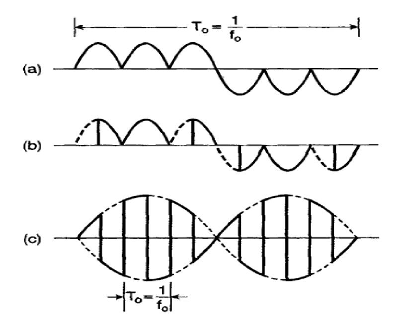
Step-up frequency conversion can be achieved by alternately switching high frequency switching devices (e.g. IGBTs, instead of thyristors) between positive and negative limits at high frequency to generate carrier-frequency modulated output.
